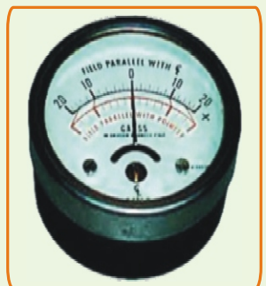
Residual Gauss meter and Field Meters in Gauss / A/cm unit of measurement
